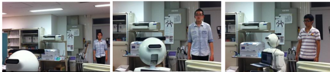
Fig. 9. The experiment result shows that the robot was able to avoid the collisions continuously when humans do not intend to interact with the robot and expect the robot to avoid the collisions.
