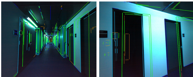
Fig. 4. These images show initial matching configurations of the Corridor sequence. ICML was able to register the lines without sample consensus matching. ICP falls into local minima on the shown setups, because some of the closest lines are false matches. The images show the initial reprojection of the previous frame prior to registration with d_{\max} = d_{\text{init}} = 64\text{px} . Green depicts matched reprojected model lines, while unmatched ones are drawn in orange. Detected image lines are cyan if they were matched and dark blue for non-matched ones.
