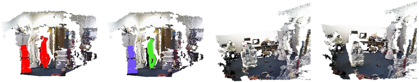
Fig. 2. (A) Foreground pixels (shown in red) are extracted from the background. (B) Connected components in the foreground image are used to find candidate objects for each frame. (C) The centroids of these objects, aggregated over all time, provide candidate correspondences which RANSAC can use to estimate an initial pose. (D) This initialization is refined with an alternating grid search on foreground objects across all frames simultaneously.
