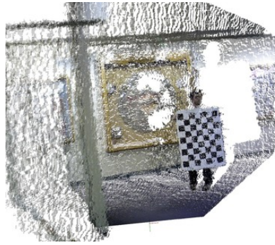
Fig. 5. Ground truth evaluation was provided by using a checkerboard to align the two sensors for each configuration. Quantitative results using this method can be seen in Figure 6.
