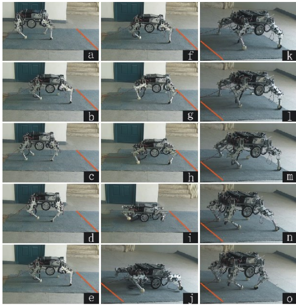
Figure 12. Sequence of snapshots of walking and mode transformation experiment. The first column shows the stage of static walking of HyTRO-I. The second column denotes the stage of transformation from the legged mode to wheeled mode, and the third column displays the stage of transformation from the wheeled mode to legged mode of HyTRO-I. Between the second and third stage, HyTRO-I rolls on wheels.
