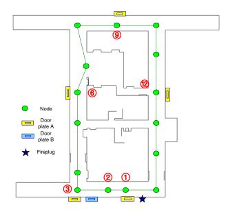
Fig. 4. Landmark (object) based map produced as a result of exploring the indoor environment.
