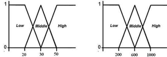
Fig. 5. Membership function for A<sub>1</sub> Fig. 6. Membership function for A<sub>2</sub>
