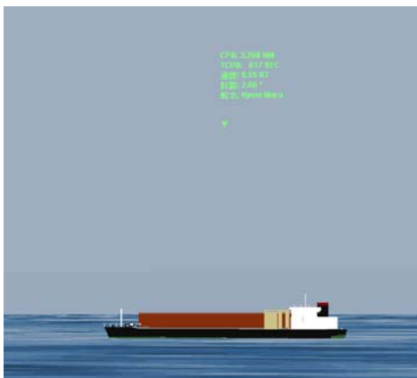
Figure 4. The example image of diplay information inscribed in green lettering. Information about DCPA, TCPA, speed, bearing, and ship name are shown above the target.
