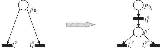
Fig. 3. Transformation from multiple source transitions to a single one.
