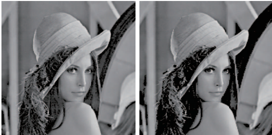
Fig. 3. Reconstructed Images ( 3 \times 1 channel). Left: Comp. Rate = 0.306, RMSE = 20.53, Right: Comp. Rate = 0.273, RMSE = 30.07
