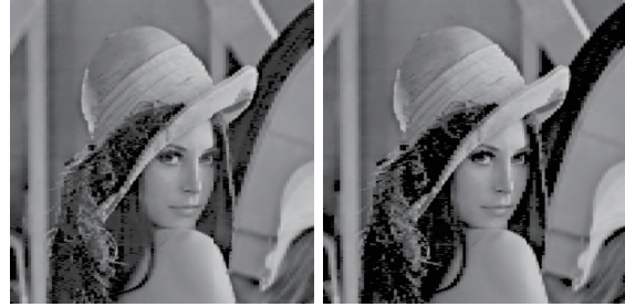
Fig. 4. Reconstructed Images ( 5 \times 1 channel), Left: Comp. Rate = 0.195, RMSE = 20.50, Right: Comp. Rate = 0.171, RMSE = 30.25
