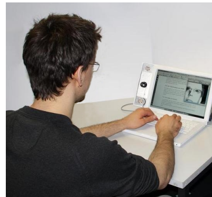
Fig. 1. Typical scenario for gaze-based interaction. The user is tracked by a remote camera, and his eye movements and gaze point are analyzed.
