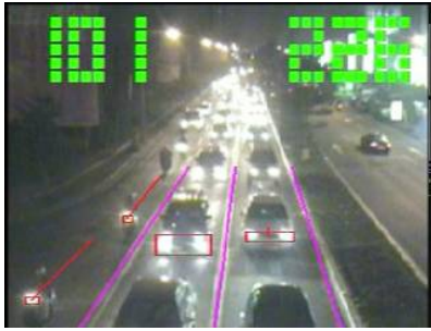
Fig. 5. Results of vehicle detection and tracking on the nighttime urban traffic scene
