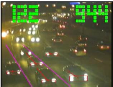
Fig. 6. Results of vehicle detection and tracking on the nighttime highway traffic scene
