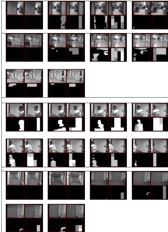
Figure 8. Examples of selected frames. Top left and top right are left and right high resolution camera frames. Bottom left is the high resolution disparity map. Bottom right is the (4×4; low resolution) tactile vocabulary pattern sent to the vibration array. Black pixels correspond to no vibrations; dark gray to vibration frequency 1; light gray to frequency 2 and white to frequency 3 (the highest).
