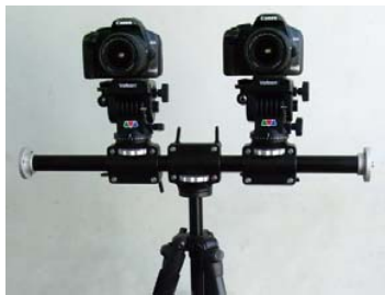
Figure 1. The binocular stereo vision system.
