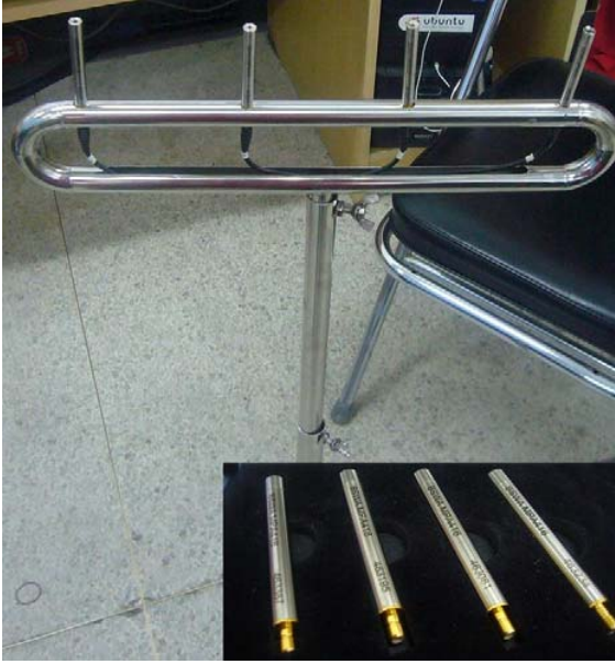
Fig.1. the experimental environment consists of four microphones and the shelf which can be applied in robot.
