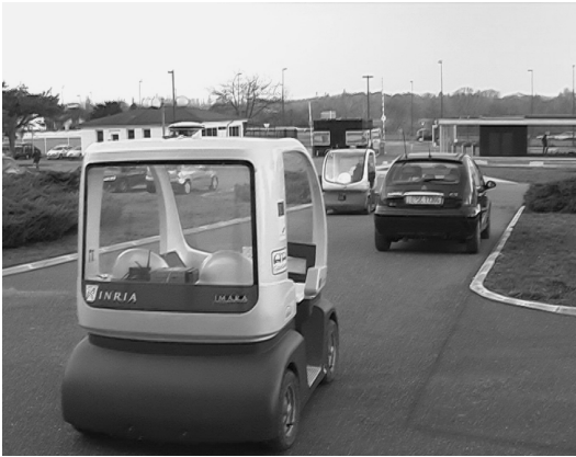
Fig. 7. Second traffic scenario: passing the stopped car is not possible due to an oncoming vehicle. After waiting until the oncoming lane is free, the driverless vehicle passes.
