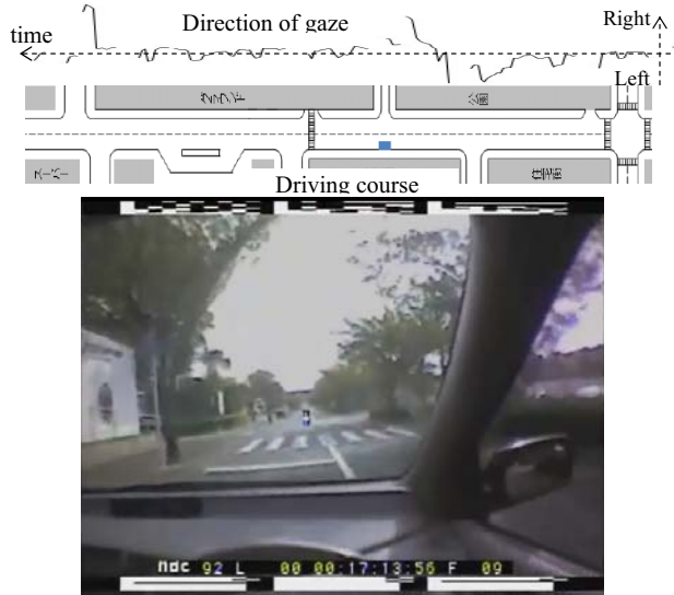
Figure 4. Road map of actual driving experiment and measured direction of gaze (upper part) and a slice of eye movement data (lower part, eye direction indicated by white "+").
