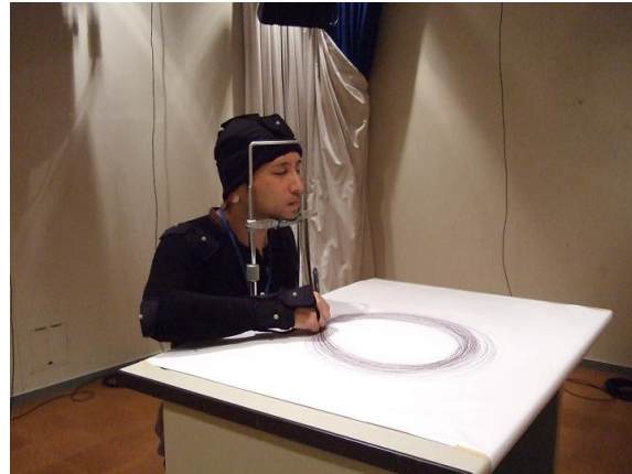
Fig. 4. Photograph of the experiment. The small silver small balls on the head, hand, elbow, and shoulder are reflecting balls for the motion capture system.
