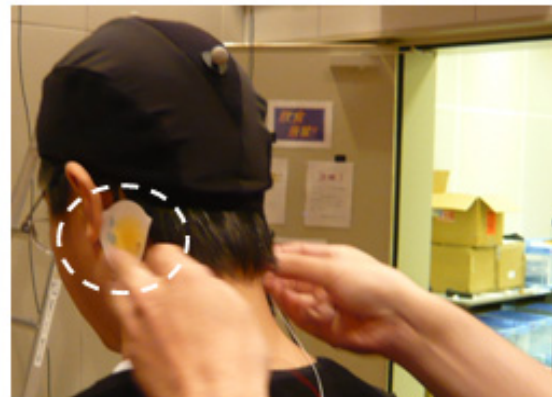
Fig. 2 GVS device of direct current is supplied to electrodes are putt on left and right mastoid tips just before the pinnas.
