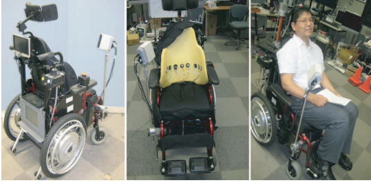
Fig. 1. Our electric wheelchair fitted with stereo vision camera (QVGA, 15fps), vibrotactile motors (5 coin-motors controlled by PWM), PC (CPU Pentium M 1.6 GHz, RAM: 1GB) and built in sound unit.
