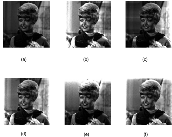
Fig. 8. (a) Girl image, the 2D-R ATs with the (b) left-to-right and (c) right-to-left directions, (d) average of images in b and c, (e) 2D-R ATs with the top-to-bottom direction, and (f) average of images in b, c, and e.
