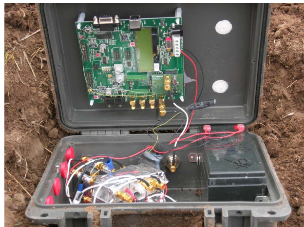
Figure 4. Revised Unit Using Commercial Wireless Sensor Node Board and Minicircuits RF Parts
