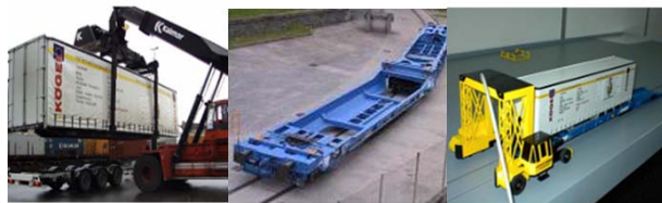
Figure 3. The three products in the project SAIL: Cranable Semitrailer (left), new pocket-wagon generation (middle), roll-On-roll-off-system (right)
