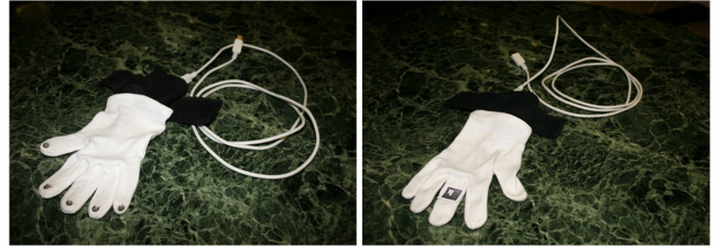
Fig. 2. Simple glove equipped with pressure sensors at the fingertips and an optical marker.
