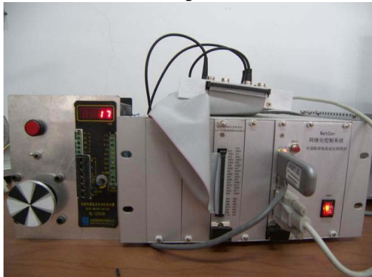
Fig. 6 the Netcontroller and the DC motor
