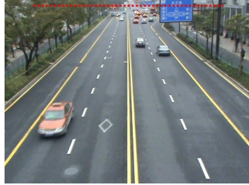
Fig. 4. The result of the nonlinear regression, the vanish point is estimated to lie on the marked line
