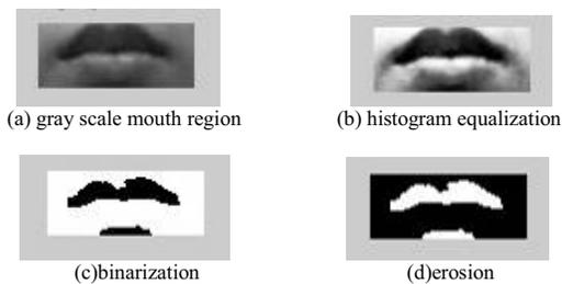
Figure 4. Process of mouth region image processing.
