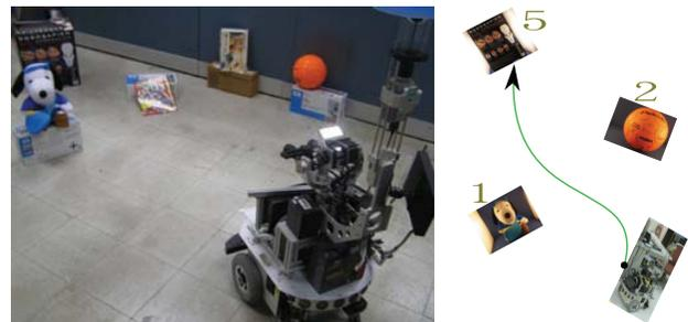
Fig. 1. The experimental setup for object recognition using our mobile robot. The robot has the knowledge of several object models, which is used for object identification and localization in an unknown environment.
