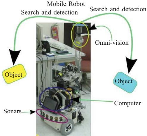
Fig. 3. The mobile robot platform used in the experiments. The encoders and the catadioptric omnivision system mounted on the top of the robot are used for object searching.
