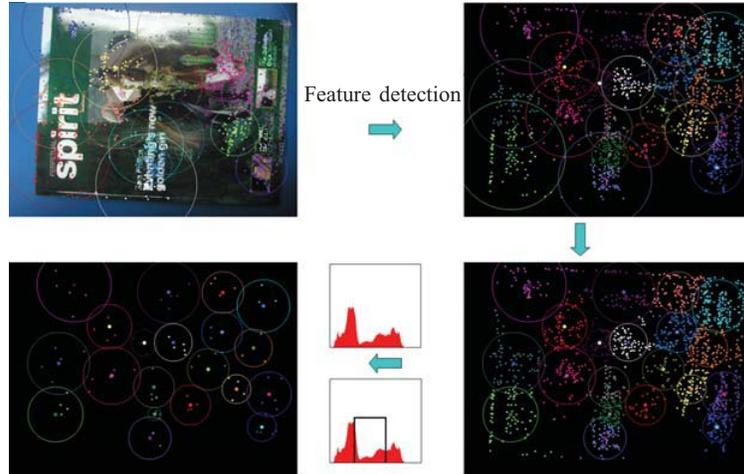
Fig. 5. We utilize the SIFT to detect the features and employ the  $k$ -means cluster. The top-left image is an object image with 2003 SIFT features. In the top-right image, only the features and the clusters are shown( $k = 20$ ). The bottom-right image is with the modified radius. The bottom-left image shows the reliable regions and choosing 89 stable features.
