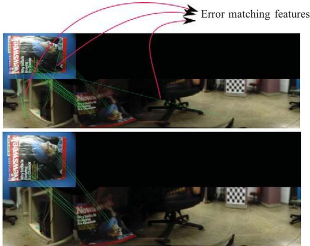
Fig. 8. The top image shows the SIFT feature matching without feature optimization. The bottom image shows the feature matching with the feature optimization. The comparison indicates the feature matching error decreased by using the feature optimization procedure.
