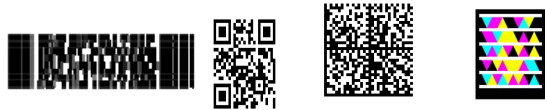
Figure 1. Examples of Barcode: (a) PDF417 code 128; (b) QR; (c) Data Matrix; (d) HCCB [11]
