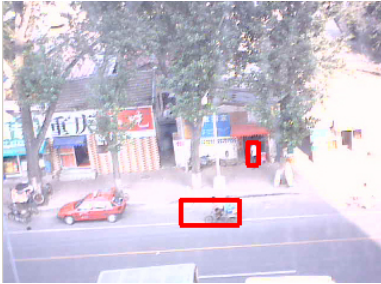
Figure 7. Result of moving multi-object detection (A passerby and a bicycle were tracking)
