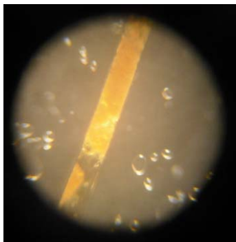
Figure 7. Channel blockage for mustard powder (x100 microscope).
