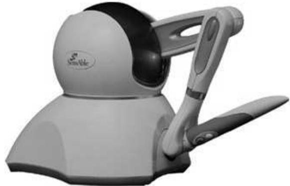
Figure (2) Three degree-of-freedom PHANToM Omni haptic device.
