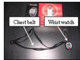
Figure 4. The heart rate monitor which consists of a chest belt and a wrist watch.
