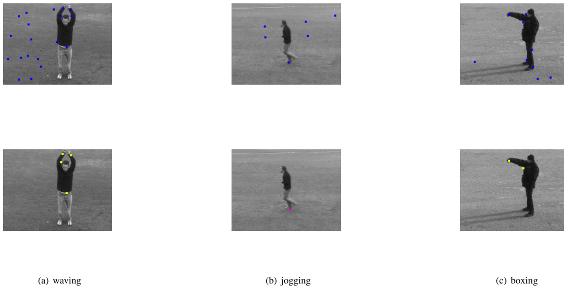
Fig. 4. Examples of STIP detected from KTH data set. The upper row are those unlabeled STIP detected under fixed spatio-temporal scales, they are represented by blue points and used as ALT input, and notice that there are some fake STIP caused by the giving fixed detecting scales. The lower row are their corresponding ALT output, i.e. the labeled results of query STIP shown in the upper row. Different colors indicating different components: pinks is associated to foot component while yellows indicating hands, and these filtered output are colored automatically in ALT.
