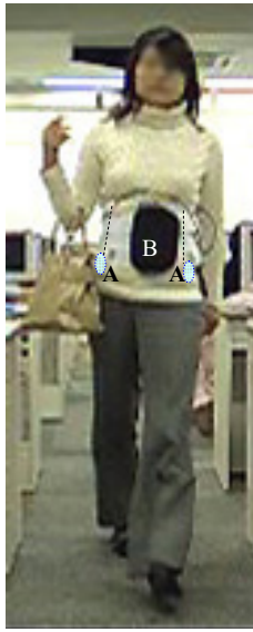
Fig. 1 The left and right hips of the subject were measured by a portable measurement system using accelerometers while walking with a bag. A is the accelerometer inside the belt, B is a waist pouch inserted with a micro-PC, memory card, and batteries.
