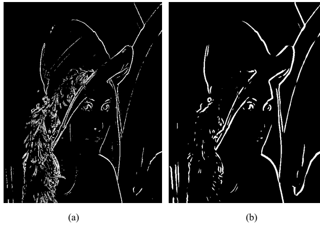
Figure 2. Sobel edge map of the original Lena image (a) and the blurred version (b).
