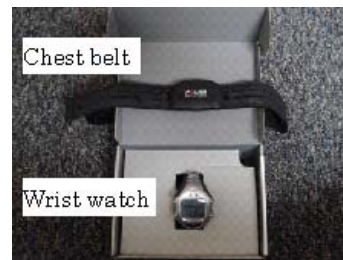
Figure 2. The heart rate monitor which consists of a chest belt and a wrist watch.
