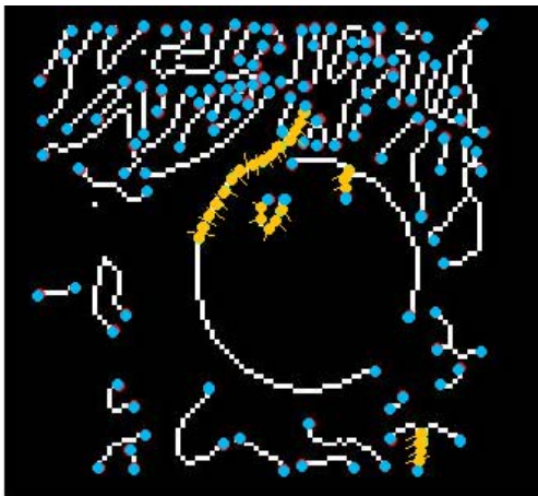
Figure 6. An intermediate stage in the algorithm while performing the morphological operations. The open ends of the open-ended chains are marked blue. The points already traversed are marked yellow with a dash.
