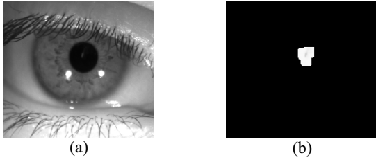
Figure 2. (a) Input image. (b) Symmetry map obtained by applying FRSD on the inverted input image. This is further used to obtain the binary map.
