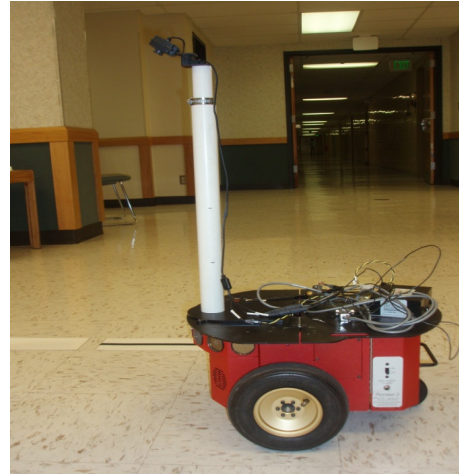
Fig. 5 Mobile robot with a mounted camera
