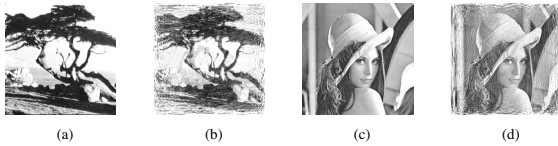
Fig. 9. (a) The tree image and (b) 2-D SQ-DFT of the image. (c) Lena image and (d) 2-D SQ-DFT of the image.
