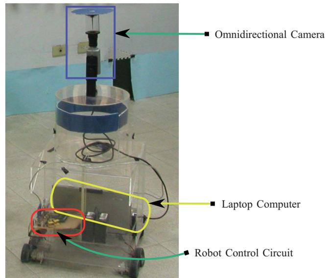
Fig. 1. The mobile robot is developed and used in this work. One omnidirectional camera is mounted on the top to detect the landmarks.
