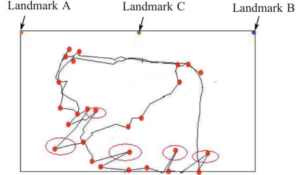
Fig. 4. The exploration global map and nodes. The lines show the feasible paths and red points are the nodes.
