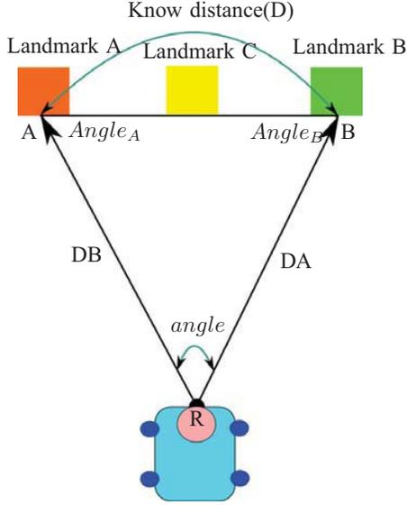
Fig. 3. The sine theorem is used to estimate the distances between the mobile robot and landmarks.
