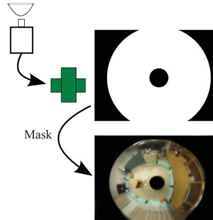
Fig. 2. The redundant region removal.
