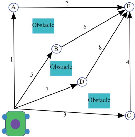
Fig. 5. An example of path planning. A - E are the nodes, 1 - 8 are the feasible paths. There are three obstacles in the map.
