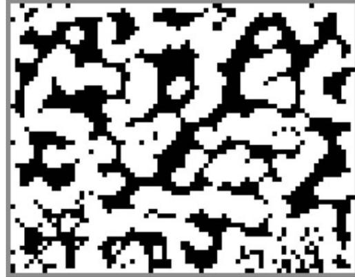
Fig. 1. Example of resulting structure after 300000 time steps for a population of Dozers. Each white pixel represents a particle and each black pixel represents an empty spot. The grey borders correspond to surrounding walls.
