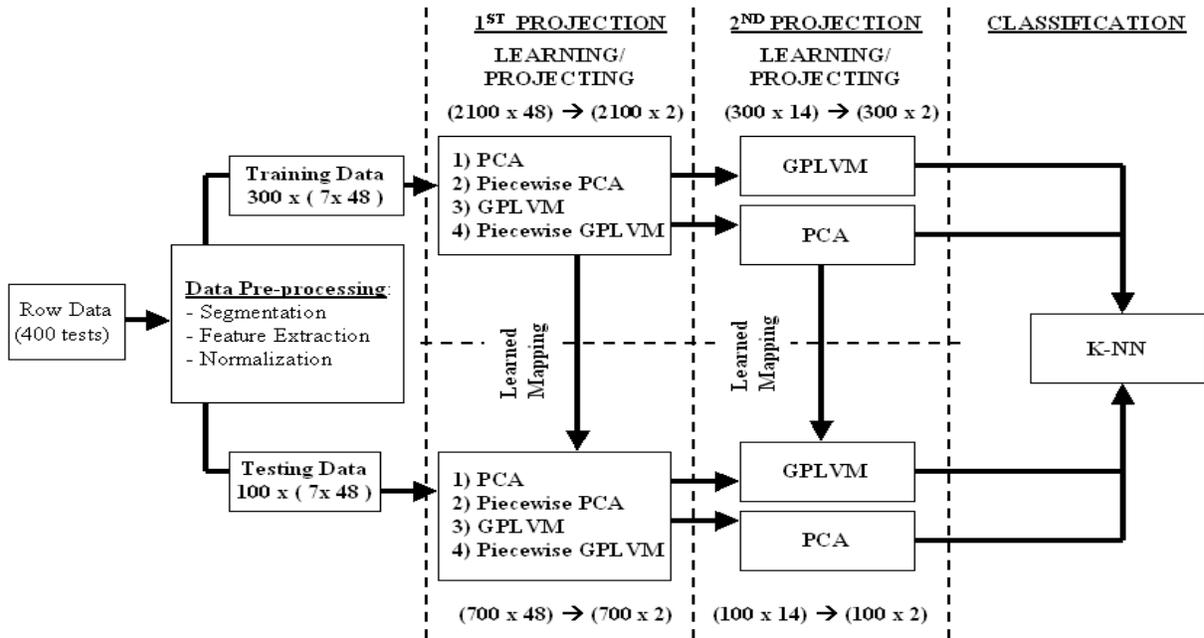
Fig. 3. Framework designed for the comparison and combination of the dimension reduction techniques, GPLVM and PCA, in fault detection applications.
