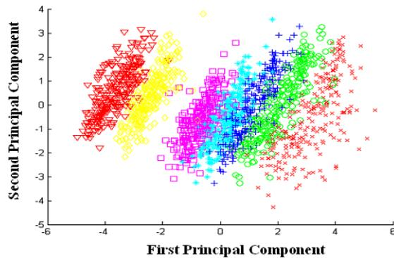
Fig. 4. Example of the result obtained after the first projection stage. The figure shows the projection obtained applying the PCA to the data. There are 2100 points divided in 7 classes.
