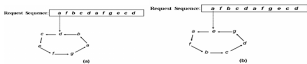
Fig. 1. Effects on accessed objects organization in disk. (a): without association rules; (b) with association rules.
