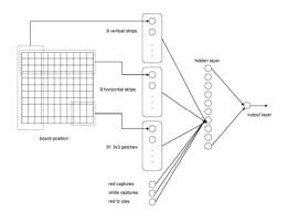
Fig 3: Structure of the neural networks used to represent evaluation functions.
