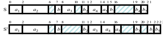
Fig. 2. Illustration of an arbitrary schedule of case2-instance in Theorem 7. The jobs are (2, 5, 1), (4, 5, 1), (2, 5, 1), (2, 5, 1), (4, 5, 1).
