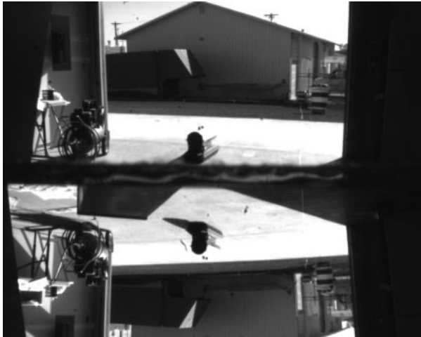
Figure 1. Raw image taken from Sleipnir's garage using single camera with a mirror box.
