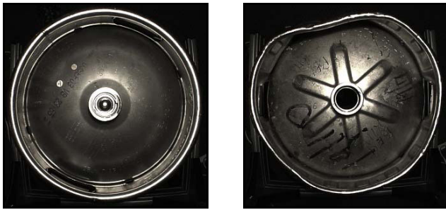
Fig. 7: (a) Ideal keg rim shape – Blefa, (b) Damaged Spartanburg keg.
