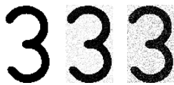
Fig. 6: Training vectors with application of random noise with standard deviation of (left to right) 0, 0.1 and 0.2.
