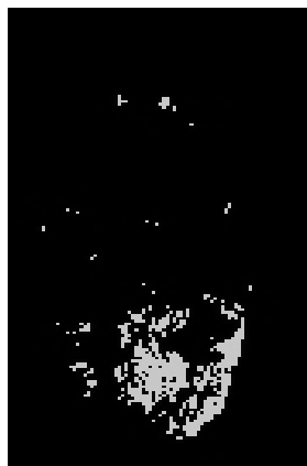
Figure 5: Intensity thresholded ROI of S05. Threshold is sixty percent of the maximum intensity.
