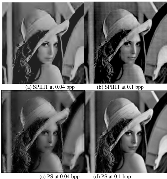
Figure 9. Visual effect comparison of the PS and SPIHT scheme
