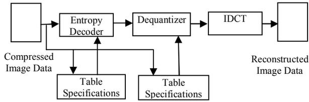
Fig. 1. DCT based decoder processing steps [3]
