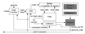
Fig. 7. Architecture of Fitness Evaluation Module with Early Termination
