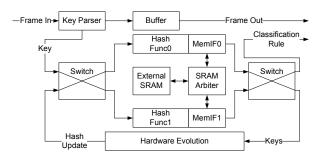
Fig. 2. The implementation of the hash function in hardware.
