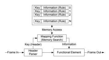
Fig. 1. A packet classifier utilizes a data base to map every incoming packet onto the proper output port.
